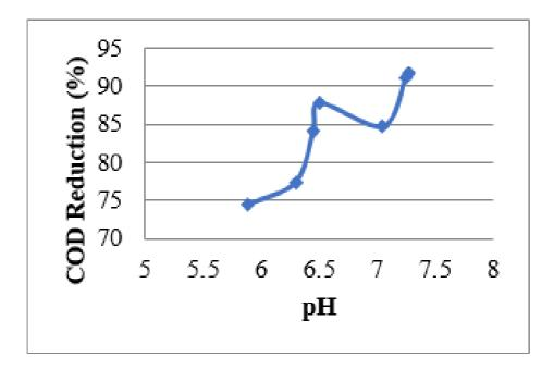
Figure 1 shows the graph of pH against COD reduction in biogas formation.
