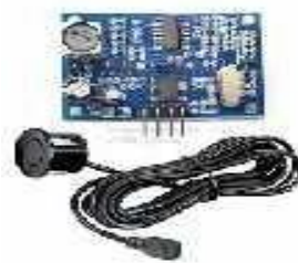
Figure 4. AJ-SR04M Ultrasonic Sensor.
